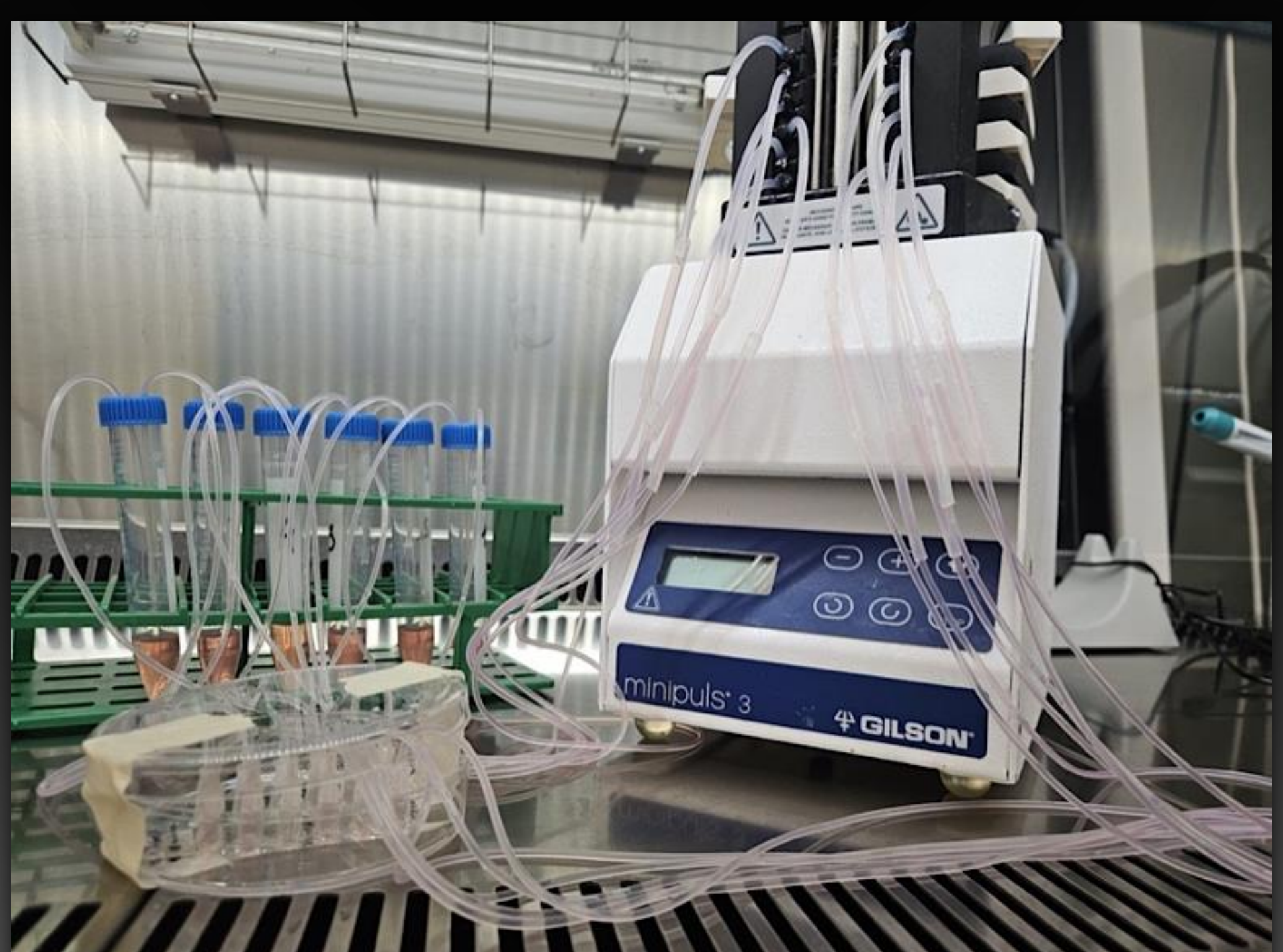
Fig. 1: Structural overview of a built 2D microfluidic system. (Walther, 2025)
